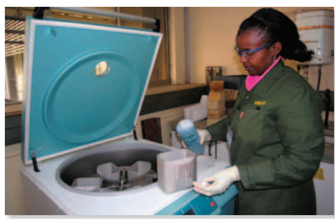
Cynthia Phiri, Mintek Laboratory Technician working with the large scale Hettich centrifuge to separate solids from leach liquor.
